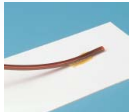
FEP is unlikely be glued, polyimide is compatible with most types of glue.
