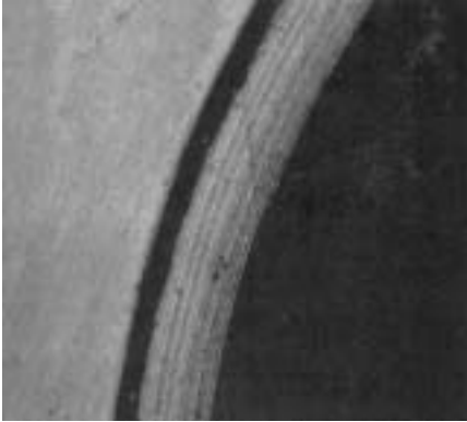
Cross section of Furukawa Polyimide Tubing (x 100)
